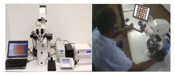
The University of Dar es Salaam Polarizing Microscope for testing the quality of face masks
